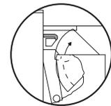
Latch retention hold is in the top latch. Retainer is released when it engages the strike. The door is in the closed position.
