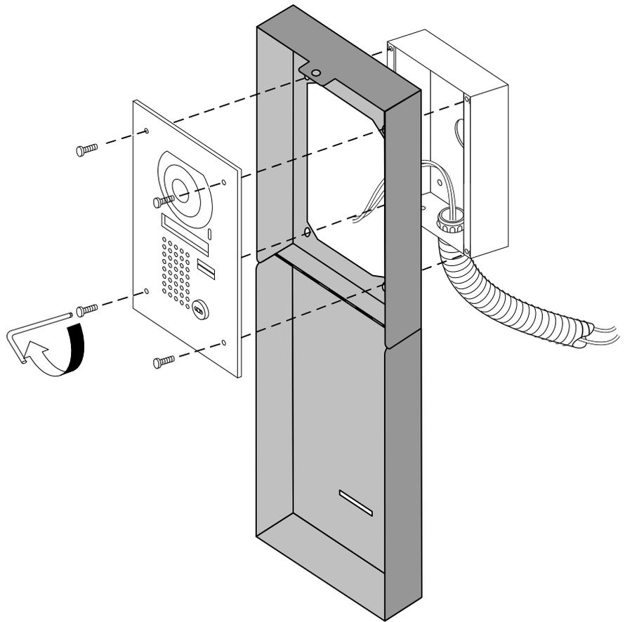
**NOTE:** Customer is to provide a security lock of their choosing to lock the panel in the closed position when the system is not in use. When in the open position, the padlock can be secured to the "L" bracket.
