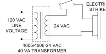
**TYPICAL ELECTRIC STRIKE WIRING DIAGRAM INTERMITTENT DUTY FAIL-SECURE 24 VAC**
