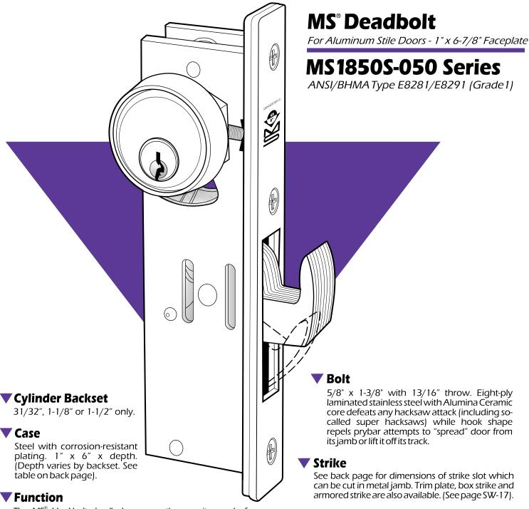
The MS® Hookbolt deadlock answers the security need of sliding glass doors in commercial, industrial and institutional buildings. The mechanism is identical to the widely used Maximum Security swinging door lock, except that the massive laminated bolt is provided in a hook shape to resist the parting motion of sliding door and jamb. The overcenter MS<sup>®</sup> locking action assures that forced entry attempts to pry the door in any direction, up, down or sideways, will be defeated.
