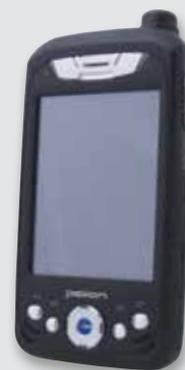
**The HHD connects with AD-Series and CO-Series locks and accessories via the USB interface**
